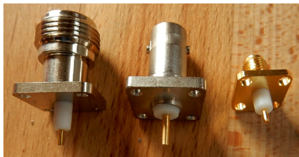
Figure 13 - Examples of suitable panel mount flanges
